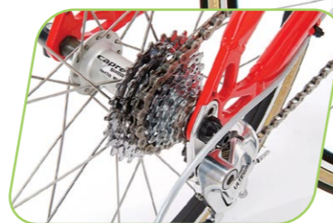
Capreo hub and freewheel combined with an Ultegra derailleur provide optimized gearing ratio on 26" wheels
